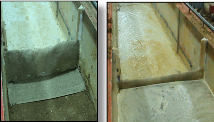
Shown Left to Right: WattleFence Before Testing, WattleFence During Testing, Flow and Turbidity Comparison*.
