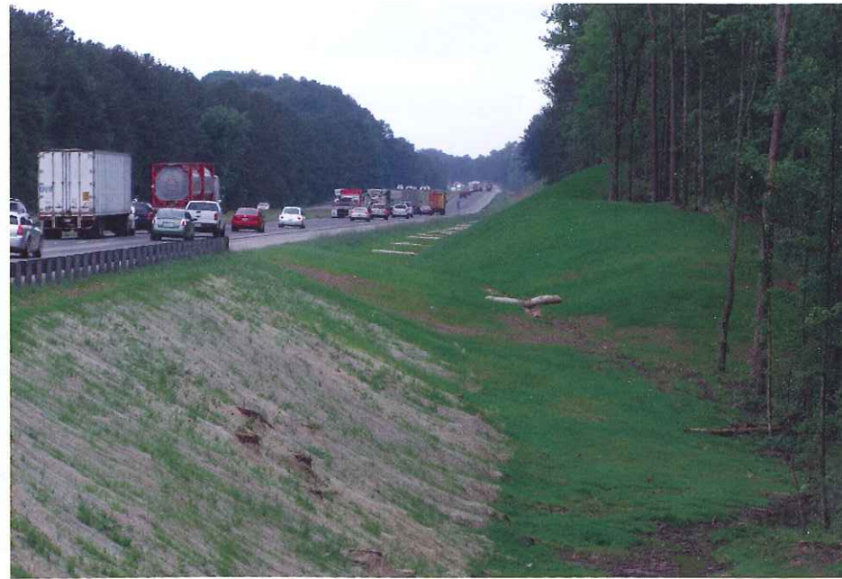
In spite of being applied five days later, the right-of-way sections receiving HydraCX 2 germinated and established grass more rapidly and thicker than the areas covered by the straw blanket.
