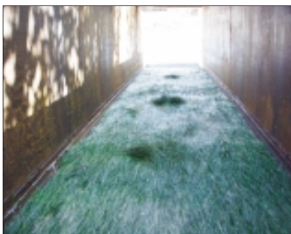
The P550 reinforced vegetation sustained the extreme 12 lbs/ft 2 (574 Pa) shear stress flow with little soil loss and NO significant damage to the P550 or vegetation.
