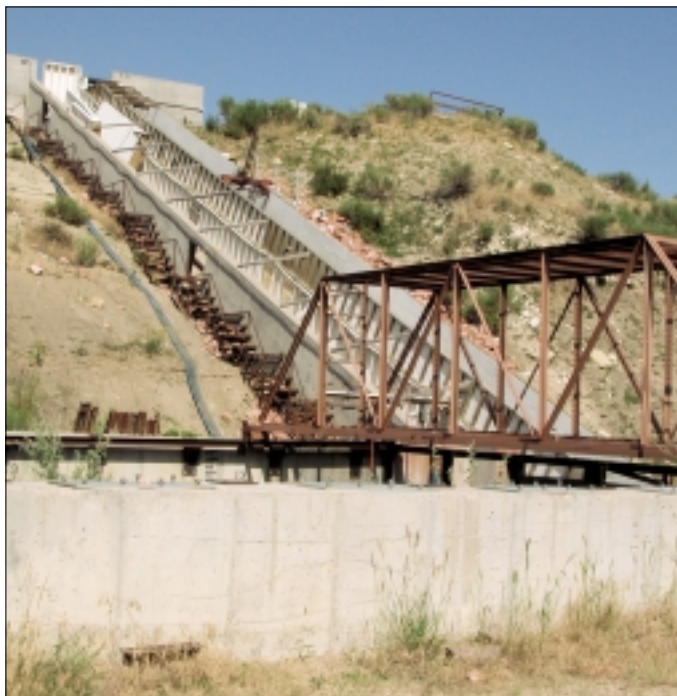
The steep flume (50% gradient) utilized at Colorado State University's hydraulics laboratory was required to generate extreme shear stress on the fully vegetated (Phase 3) Vmax 3 turf reinforcement mattings.
