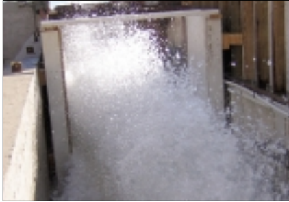
The P550 reinforced vegetation was exposed to a maximum flow generating a shear stress of nearly 20 lbs/ft 2 (960 Pa).
