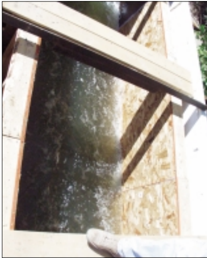
A P550 test flow generating 12 lbs/ft 2 (574 Pa) of shear stress at an approximate velocity of 20 ft/s (6.1 m/s) maximizes the 7% gradient test flume discharge capabilities.
