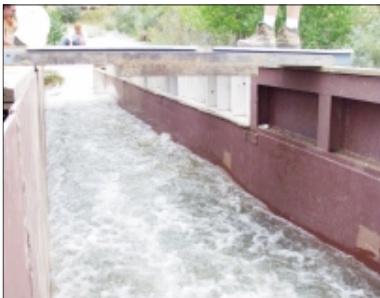
Flow generating 9.5 lbs/ft 2 (454 Pa) of shear stress with an average velocity of nearly 15 ft/s (4.6 m/s) over unvegetated P550 resulted in NO physical damage to the matting. While this value should not be used for design purposes, it does demonstrate the physical durability of the P550.
