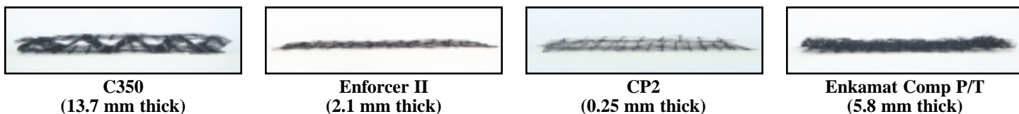
Figure 3. Composite matting’s permanent structure after organic matrices have been removed. C350’s permanent structure is significantly thicker than the other “composite” mattings and the only one able to meet FHWA TRM specification requirement for thickness (see Table 1 above).
