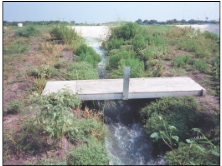
Figure 5. Flow induced shear force testing being conducted after the 90 day grow in period at the Texas Transportation Institute.
